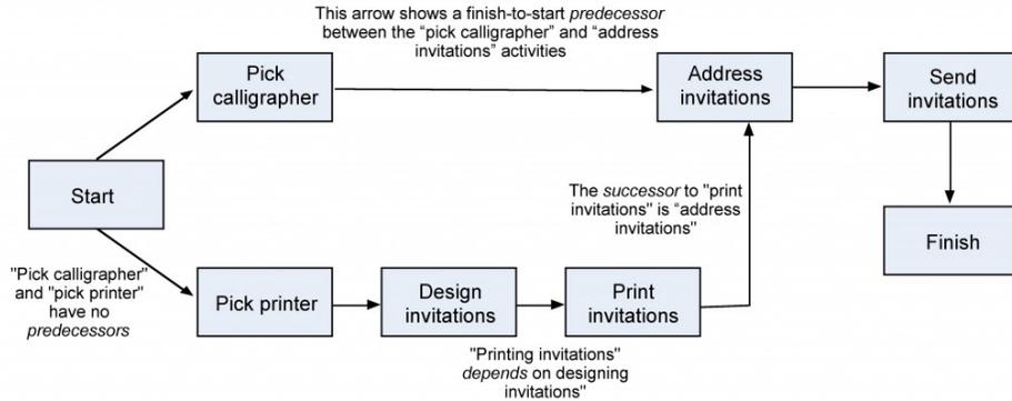
The sequence diagram is in the form of a schedule but is used to identify key scheduling information and interfaces that ultimately go into more user-friendly schedule formats, such as milestone and Gantt charts. An example of a hypothetical grid modernization related activity sequence diagram is provided below in **Figure 63**.
