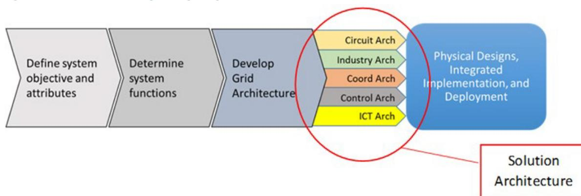
Two key parts of creating a solution architecture are identifying technologies and integrating design considerations related to system integration and data management. This technical architecture results in a chosen set of technologies that works together to meet the requirements identified to accomplish the objectives as discussed. This detailed engineering exercise results in specifications according to which the resulting solution is defined and ultimately managed and delivered.
