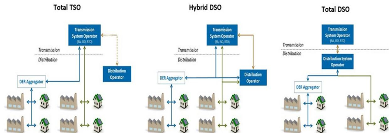
In the Total TSO model, the transmission system operator (TSO) optimizes the entire power system and oversees the dispatch coordination of all DER services and schedules; the distribution system operator
