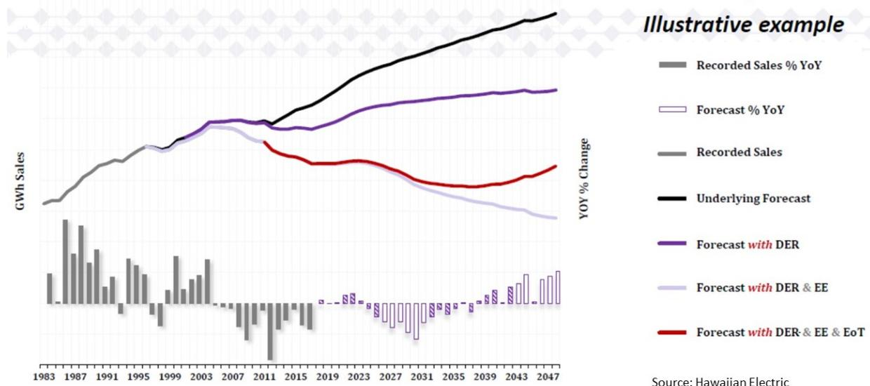
Note that customer DER is treated as an offset to customer load (net load), but if a jurisdiction has retail tariffs that allow export energy from distributed generation and storage to support resource adequacy, then these DER will need to be considered in the resource mix and not net load. The resulting aggregate net load forecast is used in an IRP analysis.
