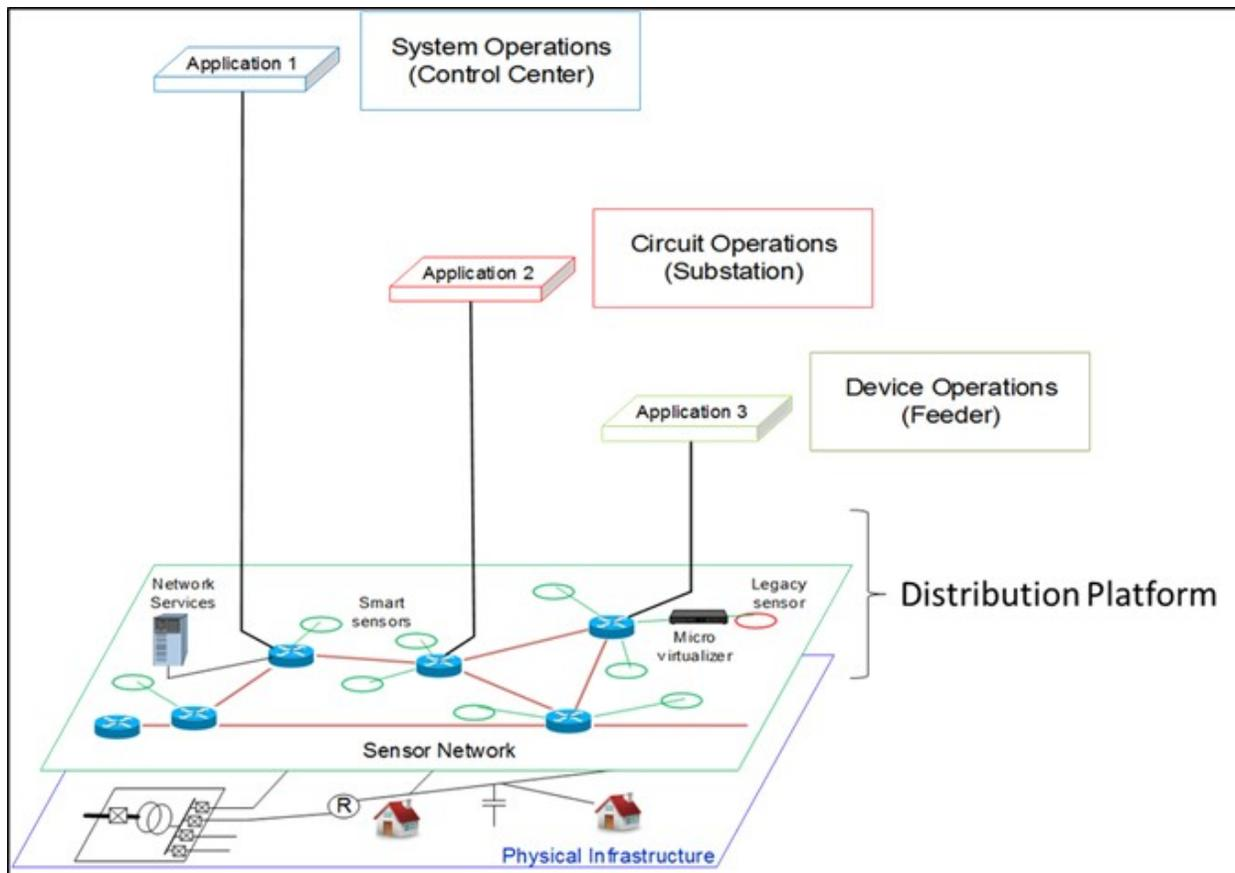
**Figure 45** illustrates how data from an AMI system may be used to support multiple operational process and analysis. Each use has unique performance and latency requirements. Smart meters can serve as sensors providing data to multiple applications.
