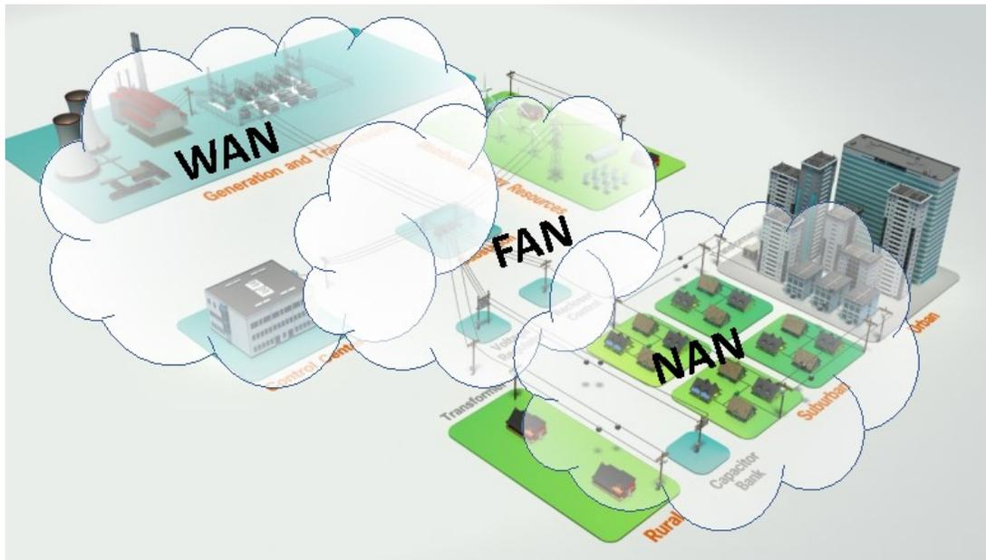
Each tier offers services that can be tailored to specific requirements of systems, devices, and applications such as bandwidth, latency, resilience, and security. Each tier also employs multiple types of communication infrastructure or media such as optical fiber, wireline, or one or more of the many wireless radio technologies available within existing infrastructure or suitable to specific locations and requirements.<sup>48</sup>
