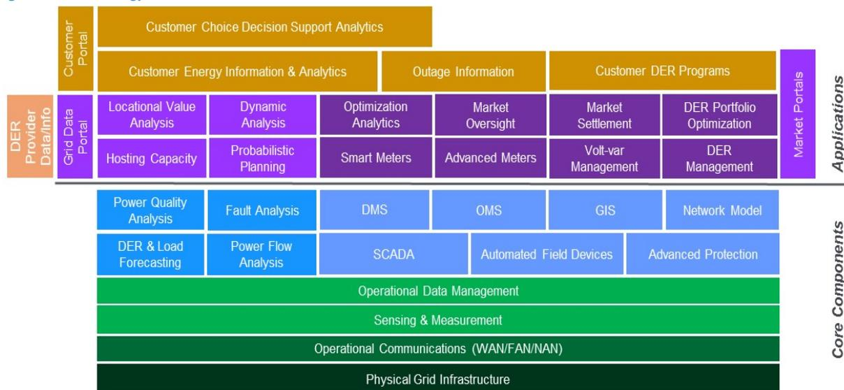
As discussed previously, it is important to consider the applications or functions needed over time to understand how to effectively build out the supporting platform. This modularization of a complex system like the distribution grid enables functions to evolve incrementally as needs dictate, consistent with the overall architecture.<sup>41,42</sup> Key properties of a platform include the ability to:
