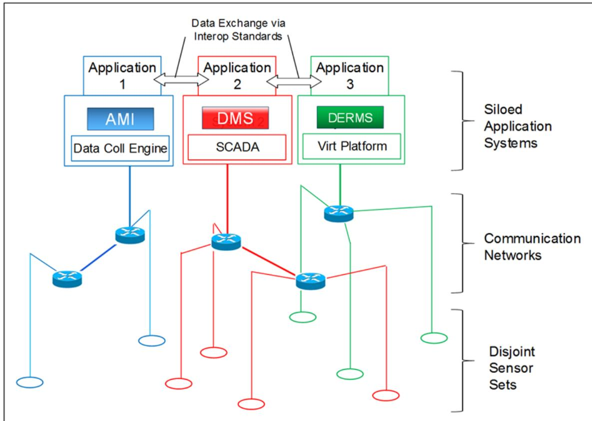
As introduced above, sensing and operational field communications for grid management and coordination can be structured as a layer of a multi-layer platform that includes the underlying electric infrastructure. Sensors can then stream data and the network can act as a publish/subscribe mechanism<sup>xxi</sup> for any authorized application, whether it is distributed or centralized, or even cloud-based (Figure 42).
